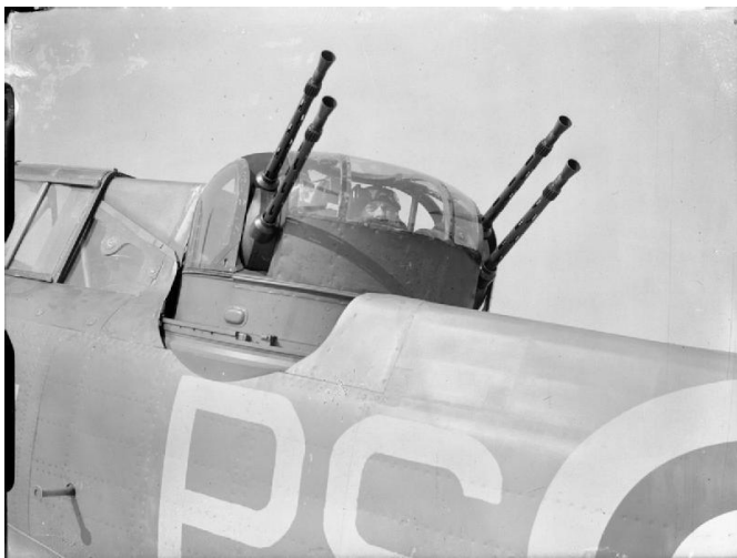
The gun turret of a Boulton Paul Defiant. The four guns fired at a rate of 80 bullets a second.
